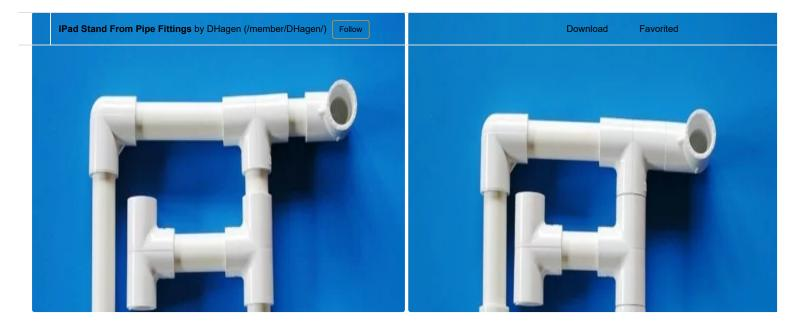
Fit the pieces together, as in the picture -- loosely at first, then snug them up. (See the second picture.) If the joints are too loose, use slightly longer small pieces of pipe.
