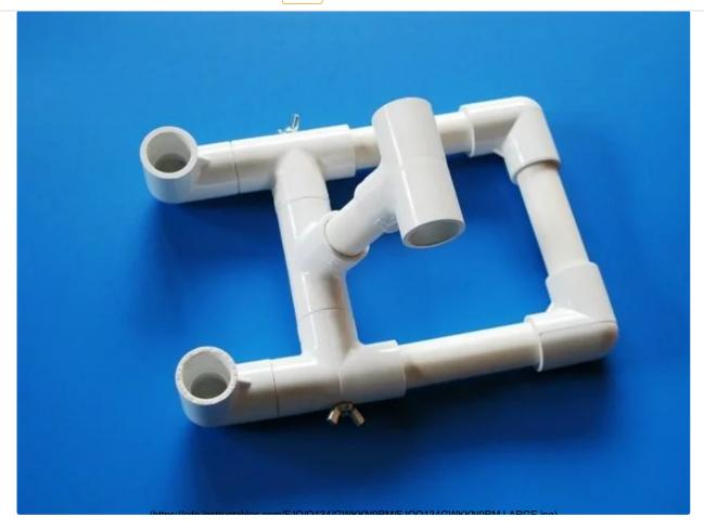
If you are worried about the iPad flopping over, add a tensioning rod. Cut a threaded rod to  $6^{1}/_{4}$ " (160 mm). The size should be 1/4" (6 mm) more than the platform width. (Your Ts may be different.) Drill a hole through the ends of the two outer Ts, push the cut rod through, and fasten with wingnuts.
