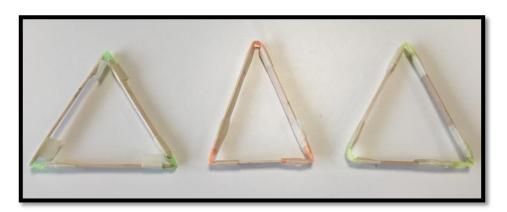
Create the joins between the pop sticks by using parts of straws. These need to be pre-cut as shown below.
