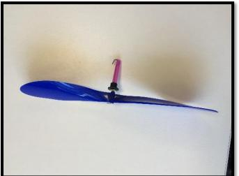
Place over the shaft and slot into the groove inside the circular part (arrow) and then tape.
