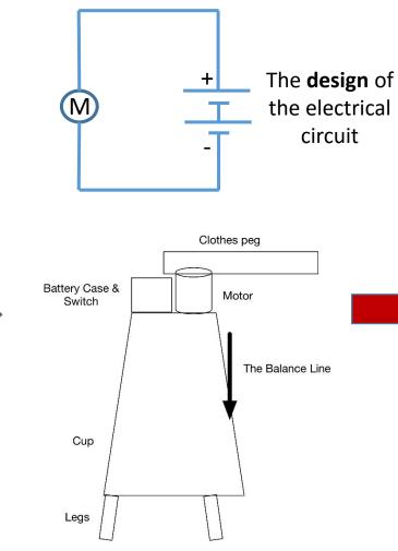
Adjusting the peg changes the balance line and rotating the peg moves the balance and generates the wiggle. How much? That is **design**!
